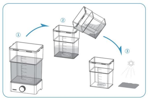
• Clean the impeller of the cleaning bucket After the cleaning bucket has been used for a period of time, the rotor at the bottom may rotate abnormally due to the sediment, then you can remove the rotor for cleaning
