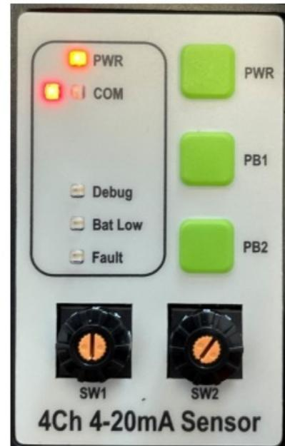
2. Press and hold the PB1 button on the CLS-4-420-TH. The RED COM LED on the CLS-4-420-TH will turn on for 1 second. Release the PB1 button on the CLS-4-420-TH.
