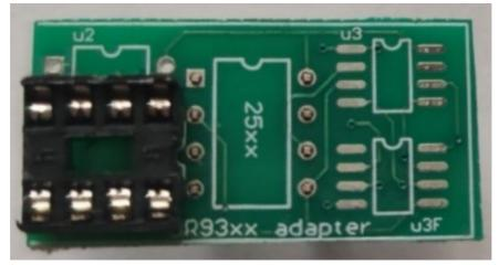
Models with F, dip inserts need to be soldered as shown above to work, sop uses U3F pads.
