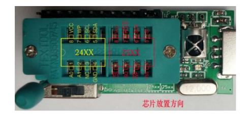
We use 16pin locking seat, every 8pin to do a series of chip burning with, the board has placed the direction of the logo. The 45xx and 93xx chips use holders, but you can't put the chips into the locking holders directly, it will burn the chips, please pay attention to it, you can only use the special adapter we delivered to realize it. Please note that there are instructions on the adapter board to put the chip into that part of the holder.
