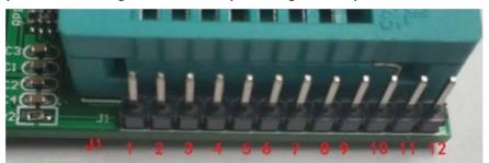
The default setting of the programmer is to short pins 1-2 of spi output J1.
