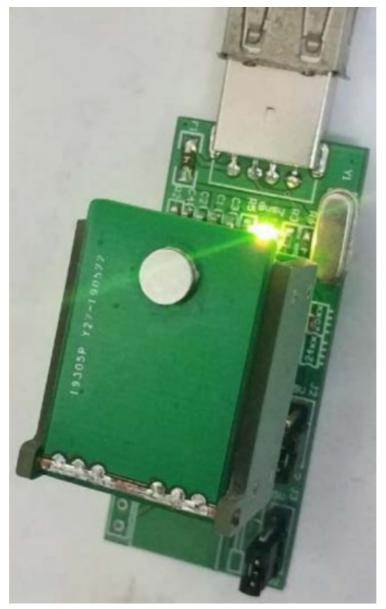
When using it, it is recommended to unplug the programmer and place the chip before plugging it into the usb port to read and write, to avoid burning the chip or usb port protection due to improper placement.
