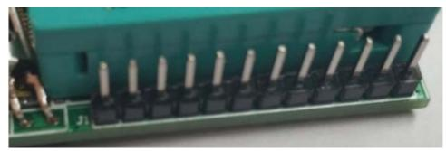
J1 pins 1 and 2 are unplugged from the jumper The following is a description of the function of J1
