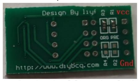
Chip pin 6, corresponding to the mark org R3R4 two resistors, R3 pull-up vcc for 16-bit mode, R4 pull-down GND for 8-bit mode chip pin 7, corresponding to the mark pre R1R2 two resistors, R1 pull-up vcc, R2 pull-down GND, this depends on the specific chip to determine, in some cases, R1 can not be soldered can also be used, 93sxx chips need to be soldered to the R2 to work!
