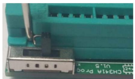
This is the read/write chip and spi pin output voltage, all through the K1 toggle to achieve different voltages back toggle switch position corresponding to the voltage identification
