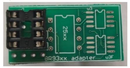
Chip types without F are soldered in the way shown above, and sop packages are soldered with u3 pads.
