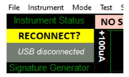
Before the instrument connects it will check the identification in the FTDI USB bridge IC, an error message will be shown if the instrument selected is not the same as the instrument connected.
