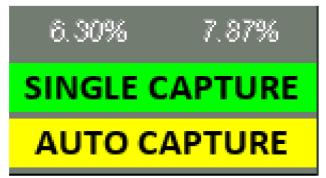
The SINGLE CAPTURE button will capture the Live Signature and it's associated voltage/resistance/frequency settings and store it as the Golden Signature for that Pin/record, once done, it will automatically advance to the
