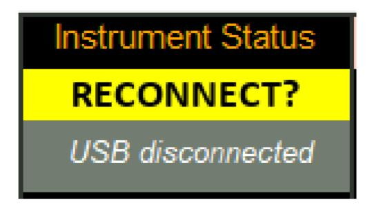
Pressing this button will connect or disconnect the instrument to EPIC. Should the instrument be disconnected, the status of this button will automatically change.
