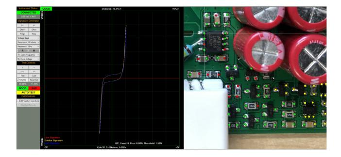
Clicking on any area of the PCB image (but not on a test point) will toggle the image from the selected view to the overall PCB image and back – this function is useful if you need to see where you are on the larger board.
