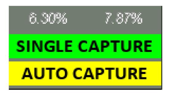
The SINGLE CAPTURE button will capture the Live Signature and it's associated voltage/resistance/frequency settings and store it as the Golden Signature for that Pin/record, once done, it will automatically advance to the next Pin/record (ready for another capture).
