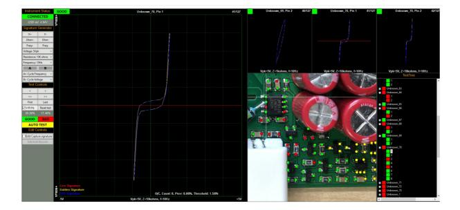
Clicking on any area of the PCB image (but not on a test point) will toggle the image from the selected view to the overall PCB image and back – this function is useful if you need to see where you are on the larger board.
