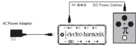
If the input polarity of the electrical device is center positive, connect the DC power cable to a polarity reversal cable (not included) and then connect the polarity reversal cable to the pedal.
