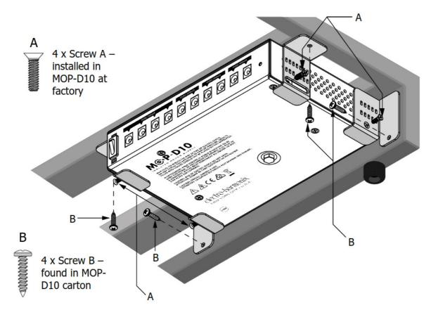
A Screws: Please note: the four A screws are installed into the sides of the MOPD10 at the factory. Remove these screws, two at a time, then reinstall while attaching the brackets.
