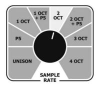
While in Sample Rate Tuning Mode, the Mainframe reads the input signal, then multiplies it by the interval selected with the SAMPLE RATE knob (see diagram) to produce the tuned sample rate of your choice.
