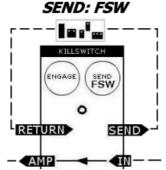
The INPUT signal only travels to the SEND jack when the FX Loop is activated.
