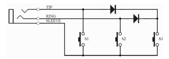
The switch connected to the TIP+RING of the external footswitch behaves like the BYPASS footswitch. Use this control to remotely switch the Superego+ on and off. This switch will also control triggers in LATCH mode.
