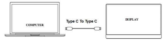
The portable display can be connected to a compatible computer using the supplied USB C cable. This must be connected to the Main USB socket on the left of the display. The computer will provide power and signal to the monitor and can be used for extended display or duplicated display use.
