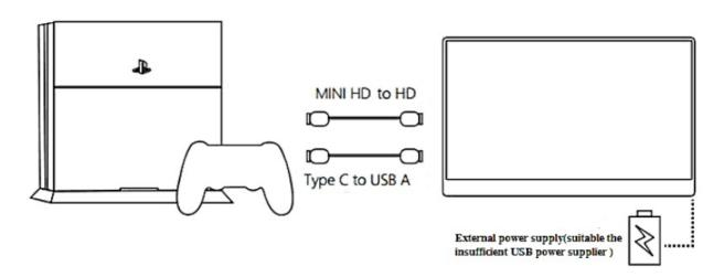
When connecting a device using HDMI, be sure to connect the power cable first, then connect the HDMI to ensure the smooth transmission of the signal.
