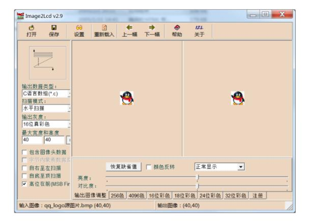
The Image2Lcd software needs to be set to scan horizontally, from left to right, from top to bottom, and with high bits in front.
