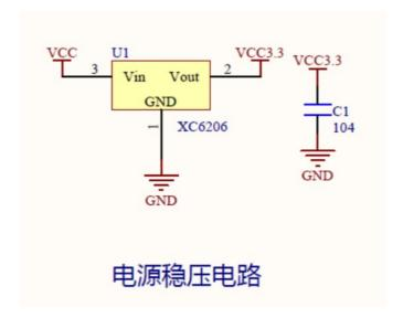
This circuit is used to stabilize the input voltage of the module, where VCC is the external input voltage, VCC3.3V is the module input voltage, and C1 is the bypass filter capacitor. VCC can be connected to 5V or 3.3V, and it is recommended to connect to 5V because only by connecting to 5V can VCC3.3 output 3.3V. If connected to 3.3V, VCC3.3 output voltage will be less than 3.3V, which will cause the backlight brightness of the LCD screen to darken.
