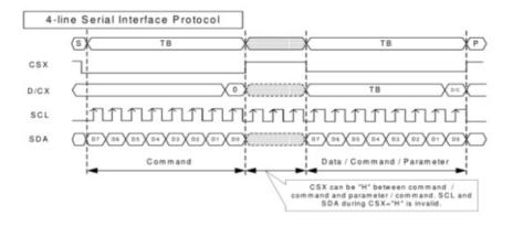
CSX is a slave chip selection, and the chip will only be enabled when CSX is at low power level.
