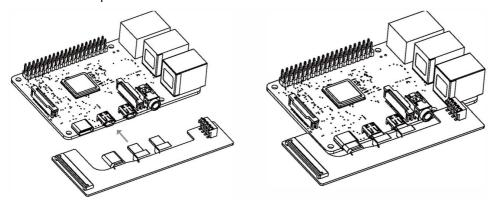
5. Insert one end of the 4 pin cable into the socket of USB expansion board, the other one insert into the socket on the HDMI expansion board.
