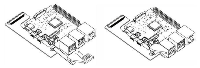
6. Put the assembled raspberry pi into the raspberry pi storage compartment, there is a magnetic base at the bottom of the compartment to fix the Raspberry Pi, Then press the GPIO adapter board with fan from top to bottom to connect the 40 pins on both sides.
