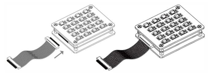
• Step 2. Insert the other end of the cable into the GPIO slot on the side of the laptop
