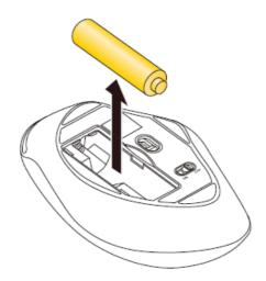
3. Insert the battery according to the instructions on the battery compartment.
