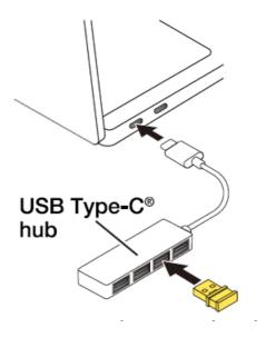
Ensure that the connector is correctly oriented to the port.
