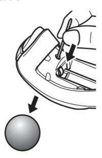
3. Use a cotton bud or similar to remove the dust accumulated on the three contact surfaces of the red ball.
