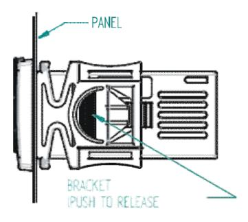
Instrument XR30CH shall be mounted on vertical panel, in a 29×71 mm hole, and fixed using the special bracket supplied. The temperature range allowed for correct operation is 0÷60 °C. Avoid places subject to strong vibrations, corrosive gases, excessive dirt or humidity. The same recommendations apply to probes. Let air circulate by the cooling holes.
