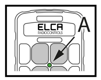
The LED [A] turns green to provide information about the radio remote control. Refer to the following table for the meaning of the LED lights. To know what to do in response to a light signal, refer to the table in paragraph 14.1.
