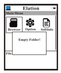
**Note:** that out of the box, the MicroSD card is blank. Make sure the MicroSD is inserted, then select Browser and press ENTER.
