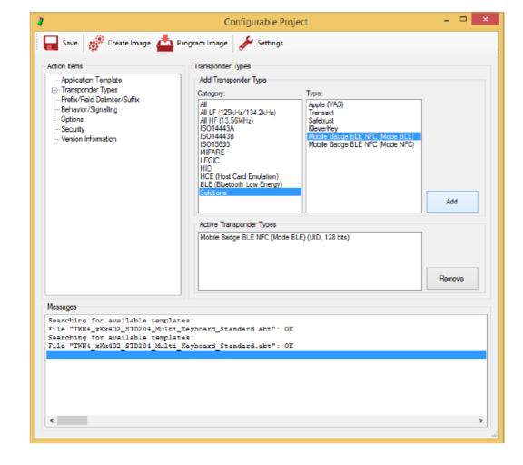
4. Using "Create Image" for compiling a new firmware image and "Program Image" button for loading it on the reader, the process of configuration is finished. The reader now supports the BLE Mode of "Mobile Badge BLE NFC" Android and iOS Apps.
