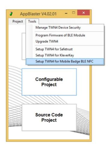
2. The current firmware running on the BLE Module will be checked in the process and the module will be reprogramed only if the firmware doesn't match the selected setup. The AppBlaster messages window will display the current firmware for the verification. In case reprogramming is necessary the process may take up to 1 minute.
