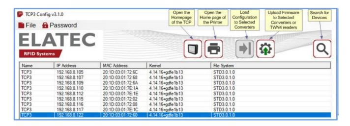
TCP3 Config is a tool that can be used to discover all of the TCP3 devices connected to the network. It can also read the configuration of the selected converter, enable editing of that configuration and can send that updated configuration back to the same converter to multiple converters.
