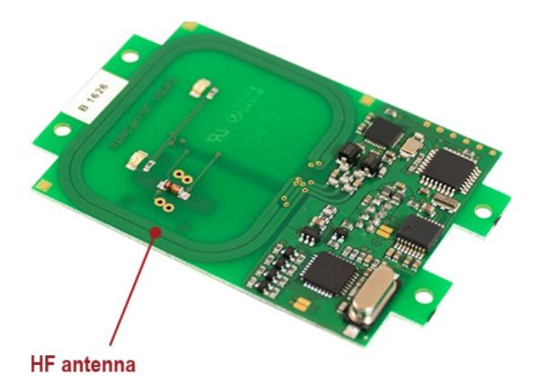
• PCB contained in TWN3 MIFARE - HF antenna (PCB air coil, integrated)
