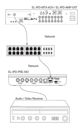
The EL-IPD-PRE-SIO enables the addition of a second amplifier to be added to an ELAN Multi-zone audio system.
