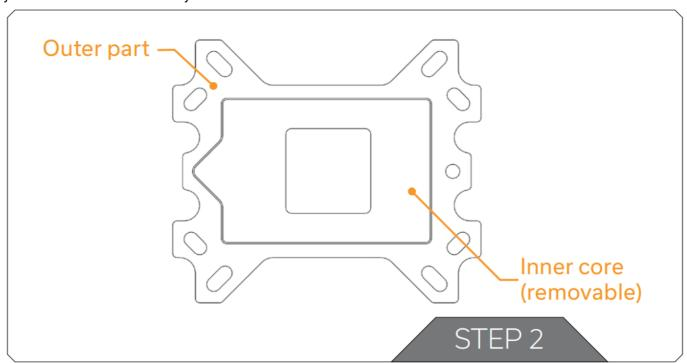
With AMD® Sockets you should use whole rubber backplate including the inner core.
