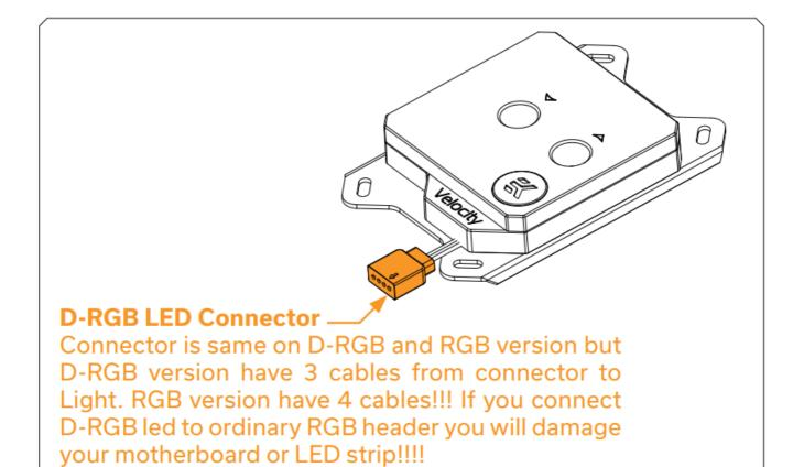
Connector is the same on D-RGB and RGB versions, but D-RGB version has 3 cables from connector to PCB; RGB version has 4 cables. If you connect D-RGB led to ordinary RGB header you can damage your motherboard or LED strip.
