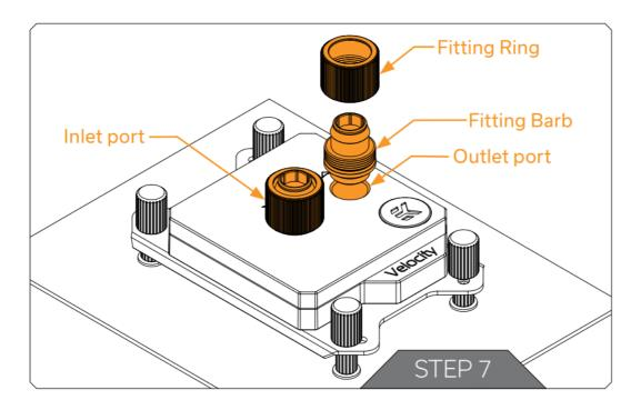
The installation of the CPU water block is now complete.
