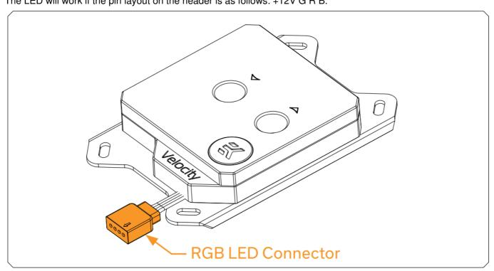
Please ensure that the arrow indicated on the connector is plugged into the +12V line as indicated on your motherboard.
