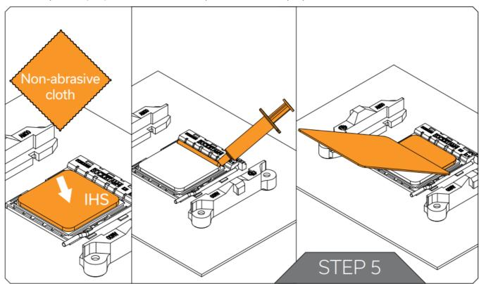
The layer of thermal compound must be thin and even in thickness through the whole surface of the IHS. Too thick application could lead to poor performance. This method applies for Thermal Grizzly Hydronaut thermal compound (3830046998477).
