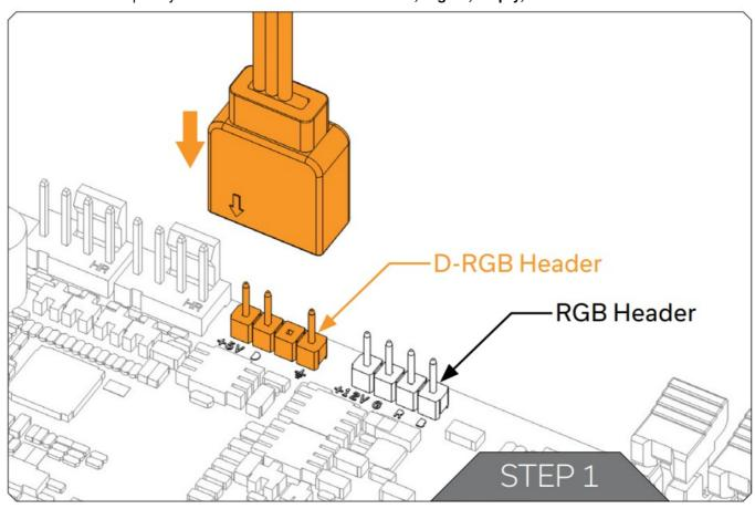
Please ensure that the arrow indicated on the connector is plugged into the +5V line as indicated on your motherboard.
