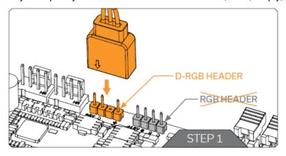
Incorrect installation or installation to a wrong header can damage the LED strip or the header itself!
