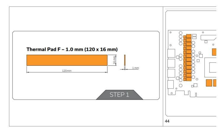
Your GPU water block comes with thermal pads that have to be cut into smaller pieces to cover all the VRM components, such as COILs, MOSFETs, and drivers.
