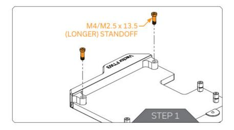
If you want to replace the D-RGB LED strip, you must remove the two (2) standoffs shown in the picture. Remove the stick out and replace the LED strip.
