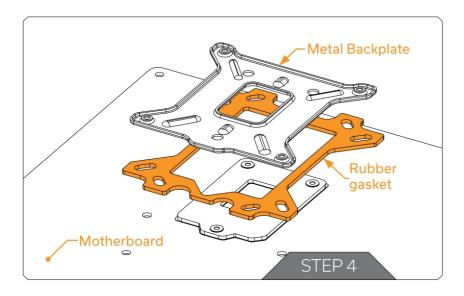
Loosely install all four Standoffs and Plastic Washers before proceeding to tighten them completely. It is mandatory for 115x,1700 and AM4 to install the Plastic Washers as they prevent damage to the motherboard PCB. Using pliers or similar tools is not recommended.
