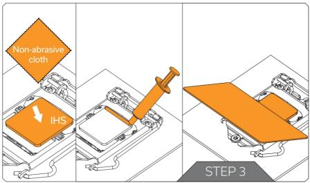
The layer of Thermal Compound must be thin and even in thickness over the entire surface of the IHS. Excessive or irregular application may lead to poor performance! This method applies for Thermal Grizzly Hydronaut Thermal Compound as supplied with all Magnitude CPU Water Blocks.
