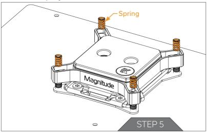
Loosely insert all four Screws before proceeding to tighten them two revolutions at once in a cross pattern. Stop when every Screw is flush with its hole inside the Frame!
