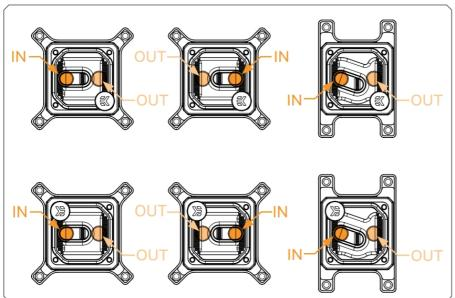
To prevent any possible incorrect assemblies the Screw hole pattern is not square. Consequently the Top, Frame, Insert, Jet Plate and Coldplate can only be rotated by 180° otherwise it will not be possible to install the Screws. The Accent, O-Ring and LED Strip may be installed in any orientation. The Insert can be rotated by following the steps on the next page.
