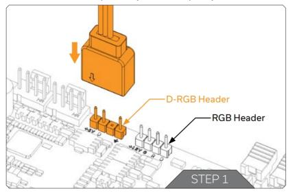
Incorrect installation or installation to the incorrect header may result in damage to the LED Strip or header!
