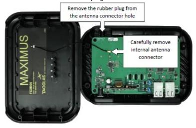
Fit the SMA connector from the inside, fit the washer and tighten the nut from the outside.
