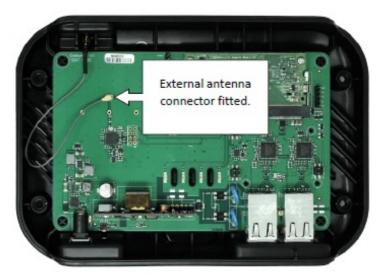
Refit the EkkoHub lid, ensuring the antenna cable is not trapped between the two halves and refit the four screws. The antenna may be mounted in a suitable location using a bracket or magnetic mount (for example Taoglas CAB.X05 (1m cable), CAB.X06 (2m cable), CAB-X07 (5m cable). Ensure that the chosen location places the antenna element in clear space.
