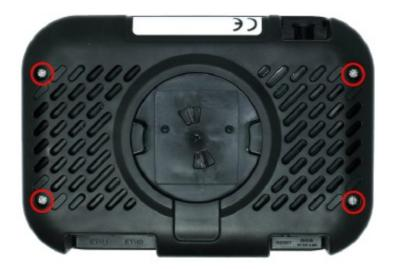
Carefully remove the lid and disconnect the internal antenna. Either remove the internal antenna, cut off the cable or fix the cable securely to the lid. Remove the rubber plug from the antenna hole in the case.
