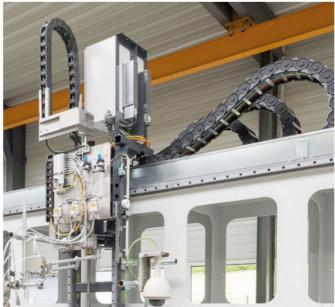
Drag chain systems are used for a wide range of applications and travel distances. EKD Systems has the right solution for every application: from self-supporting drag chains for short distances to gliding drag chains for longer distances. Our range also includes special slide shoes to reduce wear and channel systems to guide the chains.
