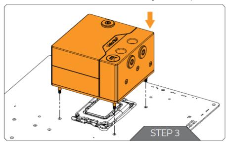
Make sure to double check the layer of the Thermal Grease before placing the water block onto the motherboard.
