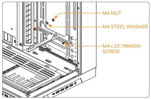
After securing the EK-Loop Angled Bracket - 140/120 mm into the chassis, you can attach the FLT reservoir. (See chapter: Attaching the Reservoir to the EK-Loop Angled Bracket)
