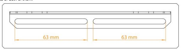
Smaller slot holes on the side allow for adjusting the position of the bracket on the radiator.
