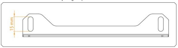
For the assembly of the EK-Loop Angled Bracket - 140/120 mm, use M4 x 4 DIN 7984 screws (as shown in the picture). Side parts already have threaded holes, so there is no need for additional washers and nuts.
