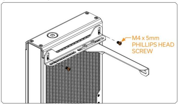
You can mount the bracket on each side of the radiator. On 280 and 420 mm radiators, the bracket can also be attached to the middle holes.
