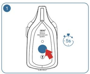
All walkie-talkies first enter the Mesh system intercom pairing state, press and hold the <intercom button> (about 5s) Until you hear the prompt "Mesh system pairing", the red light and blue light flash alternately.
