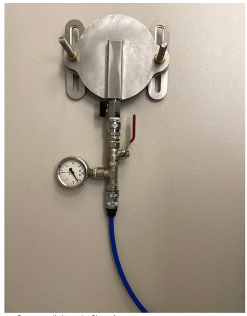
• Connect Pressure Gauge supplied to outlet Clamp A.
