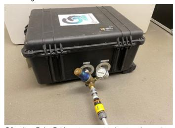
4. Connect water out hose to G2 unit at Point B (do not connect to heat exchanger).
