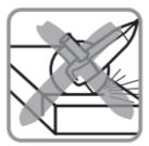
This safety guard is designed for sanding/grinding.
