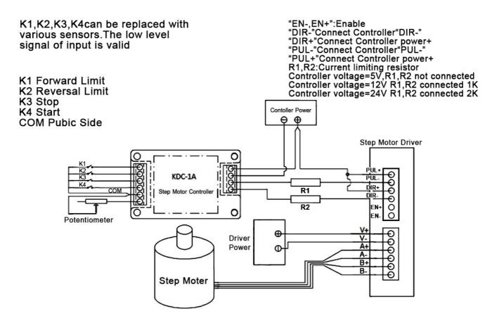
If the voltage of driver power is less than 32V, the controller and driver can share a single power supply.
