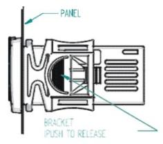
Instrument XR30CH shall be mounted on vertical panel, in a 29×71 mm hole, and fixed using the special bracket supplied. The temperature range allowed for correct operation is 0÷60 °C. Avoid places subject to strong vibrations, corrosive gases, excessive dirt or humidity. The same recommendations apply to probes. Let air circulate by the cooling holes.
