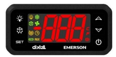
**SET**: To display target set point; in programming mode it selects a parameter or confirm an operation.
