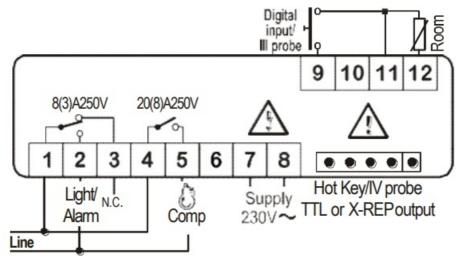
9-40Vdc supply: connect to the terminals 7 and 8.
