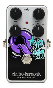
Congratulations on your purchase of the Micro Q-Tron envelope controlled filter! The Micro Q-Tron is identical to our Mini Q-Tron but in a compact pedal. The envelope controlled filter is a unique type of sound modifier in which the user's playing style controls the effect. The volume of the input signal (also called the envelope) controls the cutoff frequency or center frequency of a swept filter. As your instrument's volume increases or decreases, so does the pitch of the filter.
