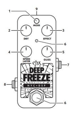
1. MODE Button Selects how the footswitch controls the effect.
