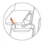
Firstly, open outward the cover of the printer cutter
