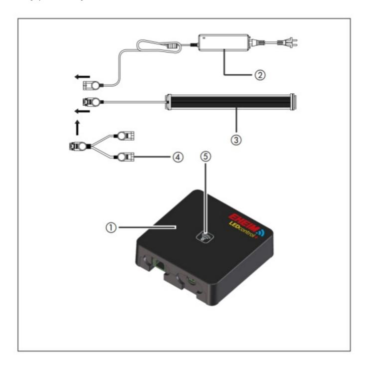
Connect the plug connectors of the EHEIM power supply ② and the powerLED+ lamp ③ with the LEDcontrol+ ①. When using an EHEIM 2-way switch ④ Article-number 4200050, multiple powerLED+ can be operated.
