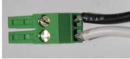
Figure 9: Correct wiring for 2-pin CT plug
