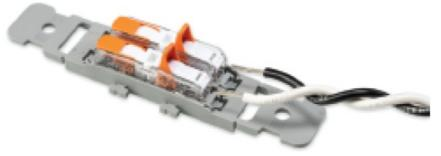
3. Lift the lever to insert the CT lead and lower the lever to secure the connection. Use one inline connector per lead wire, using two inline connectors and one carrier to extend a single CT lead.
