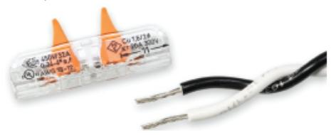
2. Remove the 2-pin connector from the CT lead and prep the lead to a strip length of 11mm (0.43 inches). Insert one of the stripped wire ends into one end of an inline splicing connector.
