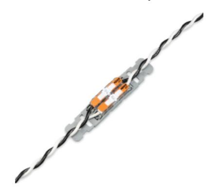
4. Strip the ends of the extension wiring to the appropriate length and connect to the other side of the inline splicing connectors in the same way. Be sure to line up black and white lead wires to the same inline connector.
