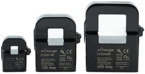
The eGauge ECS series CTs are split-core current transducers (CTs) with 36mm, 20mm, and 9mm openings. CTs are installed around current carrying conductors to measure amperage as part of a power metering solution. Thanks to the split-core design, they are easily retrofitted to existing power systems and do not require the metered conductors to be disconnected. A 333mV output means no shorting blocks are required. All ECS CTs are UL2808 certified.
