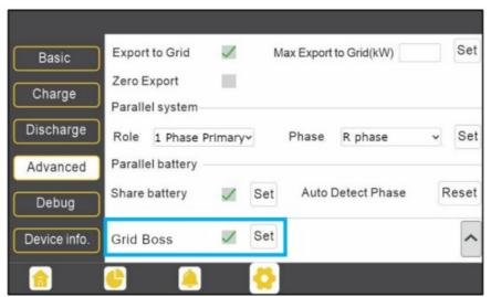
• Monitor Center: Select the "Maintenance" tab and then select "Working Mode" in the upper right area of the screen. Expand "Application Setting" and then select "Advanced Settings". Select "Enable" next to the "Grid Boss Enable" setting.
