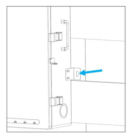
7. Remove the L-bracket and drill a hole at the marking. Use the drill bit size based on the anchor type or screw size as directed in step 3. Repeat this step for both sides.
