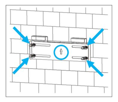
5. Using the team-lift technique, place the GridBOSS onto the wall bracket securing it to the wall.
