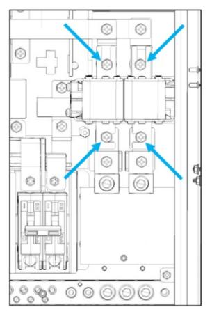
5. Set the new fuse in place. Verify the direction of the fuse matches the image below. The smaller notch open to side should be towards the grid input and the longer notch open on the end should be towards the inside of the chassis.
