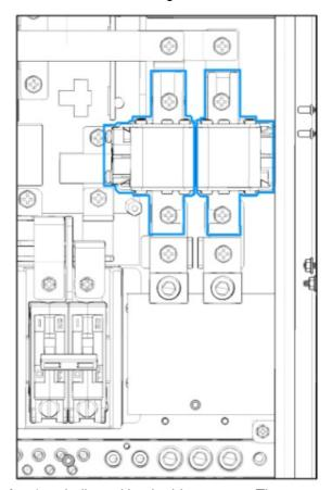
4. Remove the M6 screws (2 per fuse) as indicated by the blue arrows. Then remove each fuse.
