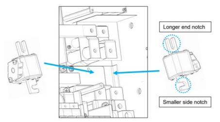
6. Reinstall the four M6 screws and tighten to 80 in-lbs. (9.0Nm).
