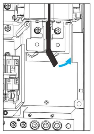
4. Install the 200A Eaton CSR25K (CSR2200N) breaker by sliding it into place, aligning the bolt holes in the breaker lugs to the holes on the busbar.
