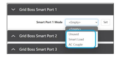
Before changing a smart port's mode, disable the port so that it does not immediately start to function. This allows the port settings to be configured while providing protection for the whole system. After fully configuring the port options, enable the port as the last step.
