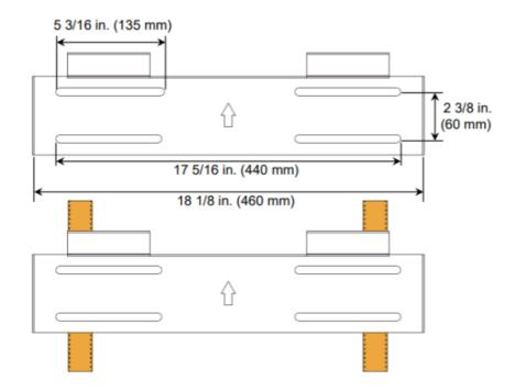
GridBOSS is designed to be wall mounted using the included wall mount bracket. It should be installed vertically on a solid, non-combustible surface such as brick or concrete. The slots on the mounting bracket can accommodate various stud spacings from 12 in. (305 mm) to 16 in. (406 mm).
