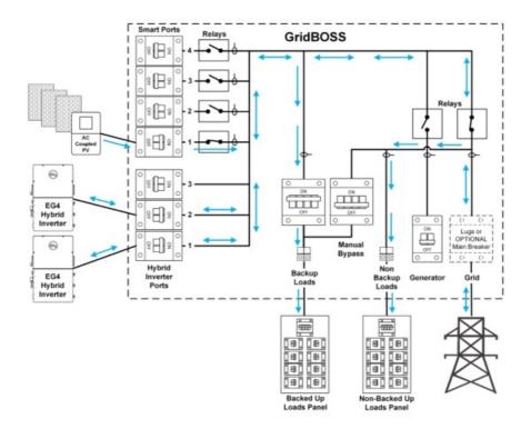
See the next page for example configurations. Each smart port is configured individually based on the device attached and usage.
