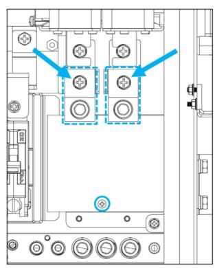
3. Before installing the breaker, adjust the position of the insulation sheet by moving the end to the right side.
