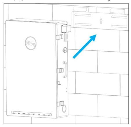
6. Temporarily mount the L-bracket to the side of the GridBOSS (located at the bottom, one on each side).
