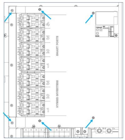
2. With the inside cover removed, locate the lugs for both line 1 and line 2 (outlined with dashed line). Remove the screw holding each lug in place then remove each lug.
