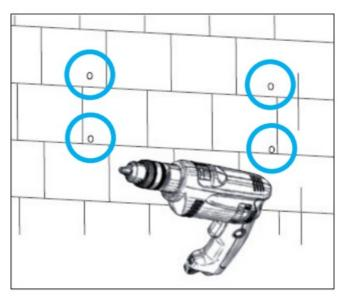
4. For concrete or brick wall installation, insert the expansion bolts into the drilled holes. Install the bracket to the wall ensuring the arrow is pointing up. Use the corresponding nuts and washers (packaged together with the expansion bolts) to affix the bracket to the wall.
