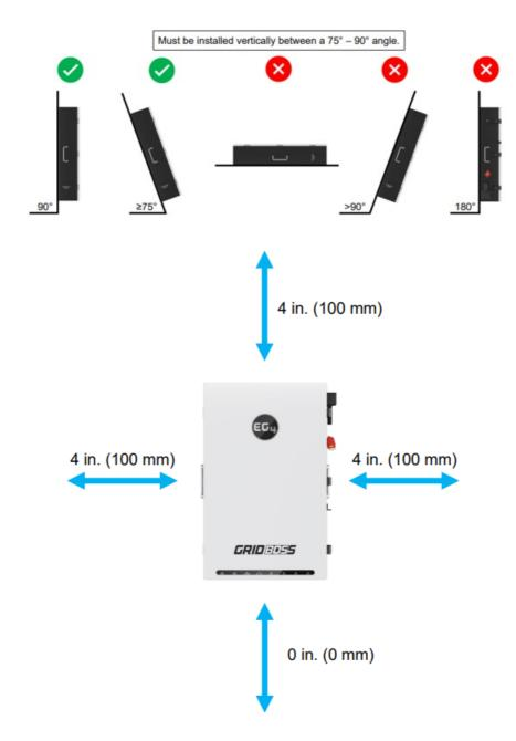
Be sure to maintain the spacing requirements shown in the image to allow access to fully open the door and to view the dongle LEDs.
