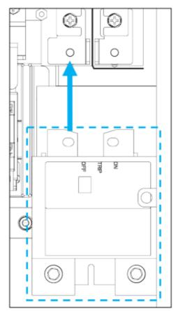
5. Using a 10 mm socket, install the two M6 screws in the busbar, then install the M4 screw that holds the opposite end of the breaker in place.
