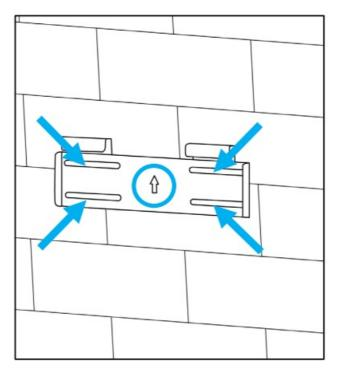
3. When installing the bracket to concrete or brick, drill 25/64inch (10 mm) diameter holes on the marks, making sure the holes are deeper than 3-3/16 in. (80 mm) when using the included expansion bolts.
