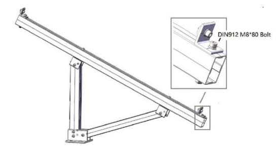
• Connect the mounting bracket to concrete anchor.
