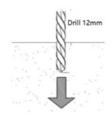
• Use the expansion screws when mounting.
