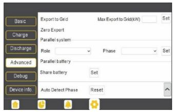
REMINDER: All setting changes for parallel inverters must be done while in Standby Mode.
