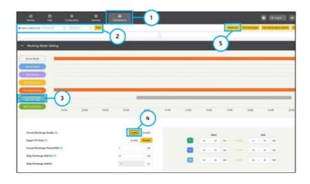
**Forced Discharge:** Forced discharge prioritizes battery power for powering loads and grid sell back.
