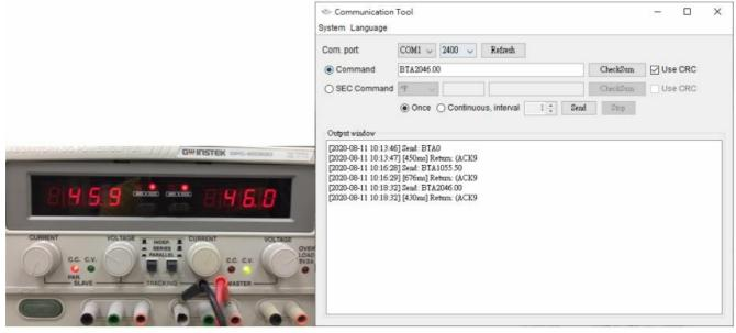
8. Change Power supply's voltage. Send command "QPIGS", compare the return's value and actual battery's
