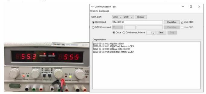
7. Adjust the power supply to 46V and send command "BTA2046.00", the Inverter returns (ACK.
