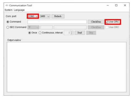
5. Send command "BTA0", the Inverter returns (ACK.
