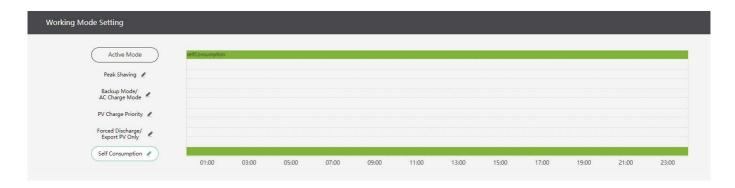
The station will default to Self-Consumption mode. The order of priority for powering loads is Solar > Battery > Grid. The order priority for solar power is Load > Battery > Grid which creates an ideal scenario when needing to prioritize solar power generation over other types of power.
