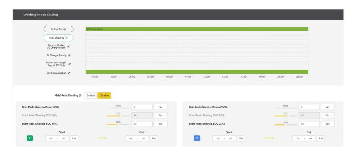
When setting the station into this mode, the inverter will use peak-shaving to avoid peak demand charges from the grid. The user will be able to configure the system to pull limited (or no) power from the grid for charging batteries or powering loads by setting maximum power in kW, according to SOC/voltage, and by setting time of use. Upon selecting the working mode, the system must be configured using the settings listed below:
