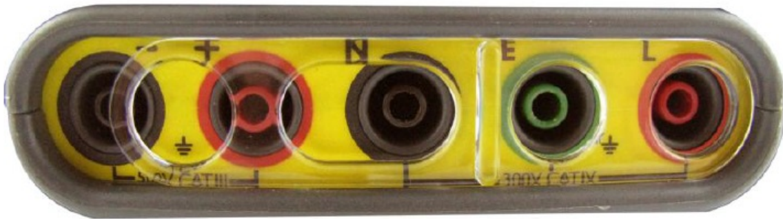
Fig.2 Interlock in position for RCD & Loop testing
