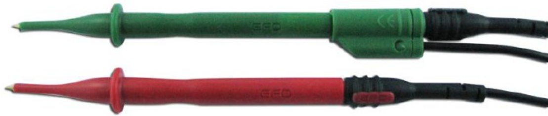
Fig 3. Prods in 2 wire testing configuration
